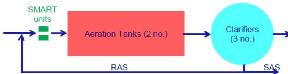
Figure 2.1: Outline HYBACS Flow Schematic
